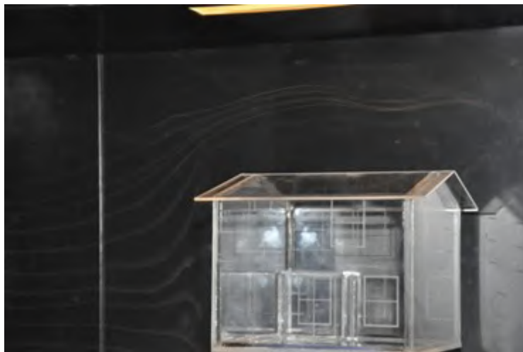
Figure 9. Aerodynamic performance of the scaled model within the wind tunnel.
