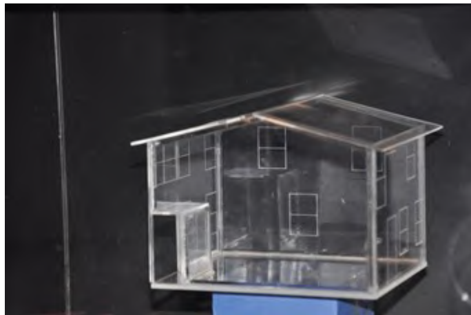
Figure 4. Physical representation of a typical social housing unit in Mexico within the wind tunnel.
