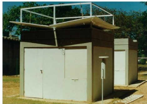
Fig. 1: The test facility (experimental and reference cells) with the continuous evaporative passive cooling system.
