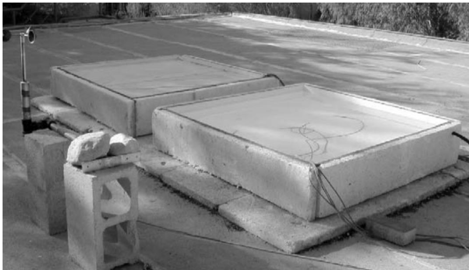
Fig. 2-3 Configuración experimental, módulo con toallas lado izquierdo. Fuente: Tang, R. y Etzion, Y. (2003) Comparative studies on the water evaporation rate from a wetted surface and that from a free water surface. Building and Environment 39 pp. 80.
