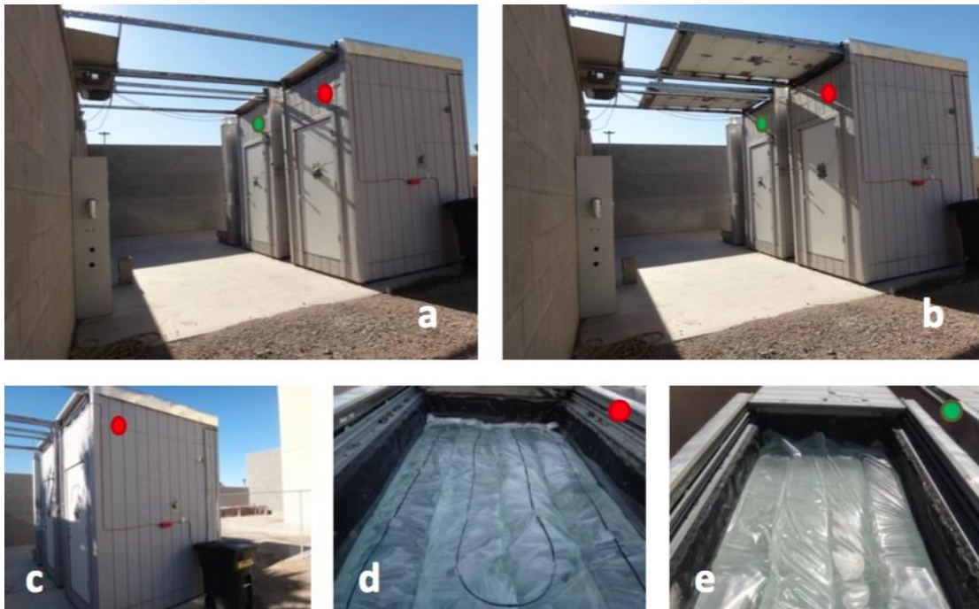
Fig. 2-14 Módulo experimental y módulo de control. Fuente: Fernández, A. (2014) Characterization of a Thermal Comfort in a passively cooled building located in hot-arid climate. Proceedings of 8th Windson Conference. Counting the Cost of Comfort in a changing world. Londres.
