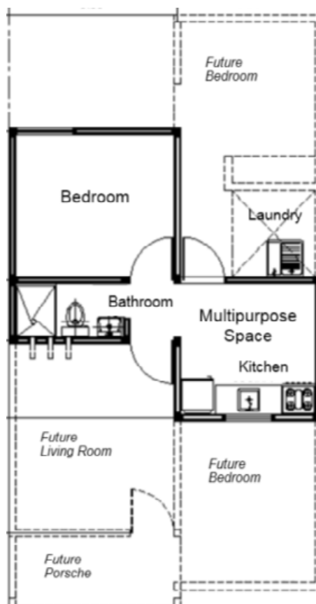
Figure 3. R1A model of affordable housing was the most built in Colima up to 2006. Floor Plan.
