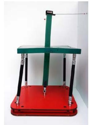
\*SD 63 Slab connection - column subjected to bidirectional lateral loads\*
