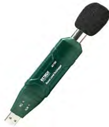
Figura 5.12 Sound Level Datalogger Extech, modelo 407760.
